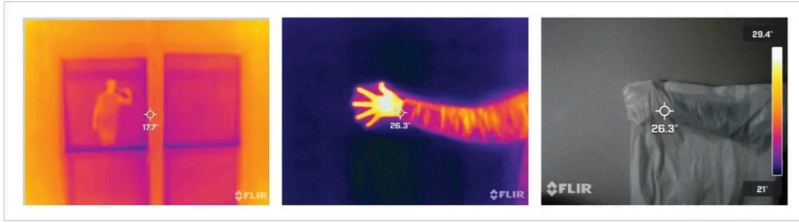
Figure 3. Thermal cameras can see reflections in glass and through thin plastic sheet/film
