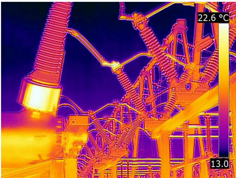
Figure 2. Radiometric thermal cameras calculate temperature
